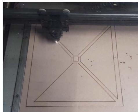
Figure 6: The process of cutting the flat view frame with a laser cutter.
