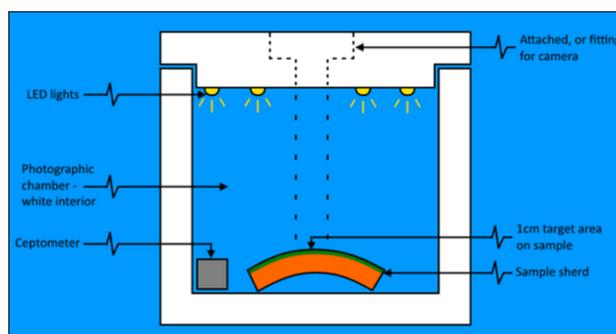
Figure 1: (Above) The Initial 2D design for the light chamber.
