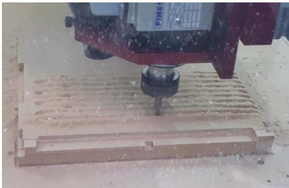
Figure 5: The process of carving the West panel with a rotating drilling machine.
